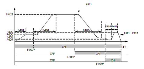
The door close process in distance control is as follows:
