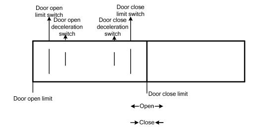
Set the parameters in group F3 related to speed control correctly. Set the deceleration switches and limit switches properly. The door open running curve in speed control is shown as below:
