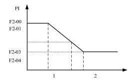
The speed dynamic response characteristics in vector control can be adjusted by setting the proportional gain and integral time of the speed regulator.
