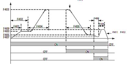
The door close process in speed control is as follows:
