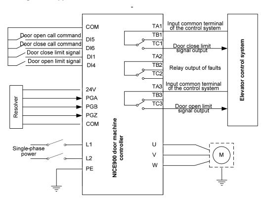
In this mode, if the limit switches are valid, the output is the door open/close limit signal output 0 rather than the pulse.
