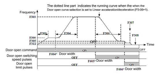
The door open process in distance control is as follows:
