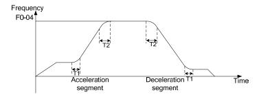
T1 stands for F5-07, during which the slope of the output frequency change (that is, speed change rate) increases gradually. T2 is stands for F5-08, during which the slope of the output frequency change reduces gradually to low-speed frequency. Between T1 and T2, the slope of the output frequency change keeps unchanged.
