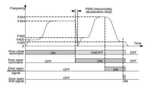
If the door is hindered during close, the controller decelerates to stop with "Abnormality deceleration time" set in F5-00. When the door is re-opened, the controller starts at a low-speed for door open, and runs at a high speed after the door open startup low speed running time in speed control set in F3-02. After the door open deceleration signal becomes valid, the controller runs in a low speed until door open limit and outputs the door open limit signal.
