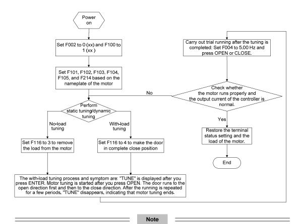
Ensure that the encoder signals are normal before tuning. If the door runs to the close direction and locked-rotor occurs after tuning is started, it indicates that the running direction of the motor is abnormal. In this case, exchange the motor or encoder wiring.
