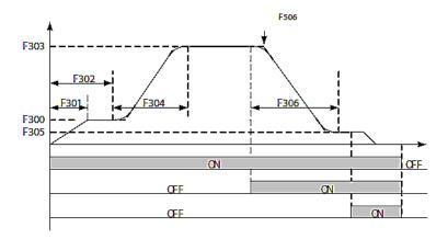
The door open process in speed control is as follows:
